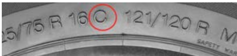
FIGURE 3: Size and Service Description of an Example C-Type European Commercial Metric Tire
